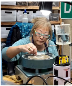
Lisa taking the first step in preparing the stone to put it on a Dop stick. The first side must be flat to apply it on the dop stick.
